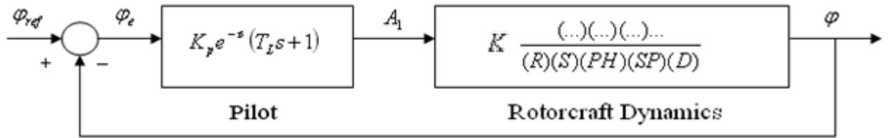
Figure 3. Bandwidth roll control block diagram
