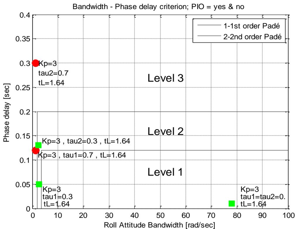
Figure 8. 1<sup>st</sup> order Padé approximation vs. 2<sup>nd</sup> order Padé approximation
