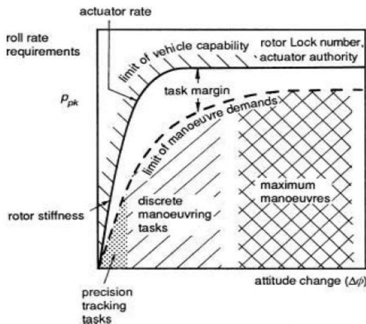
Figure 2. Roll rate requirements as a function of maneuver amplitude
