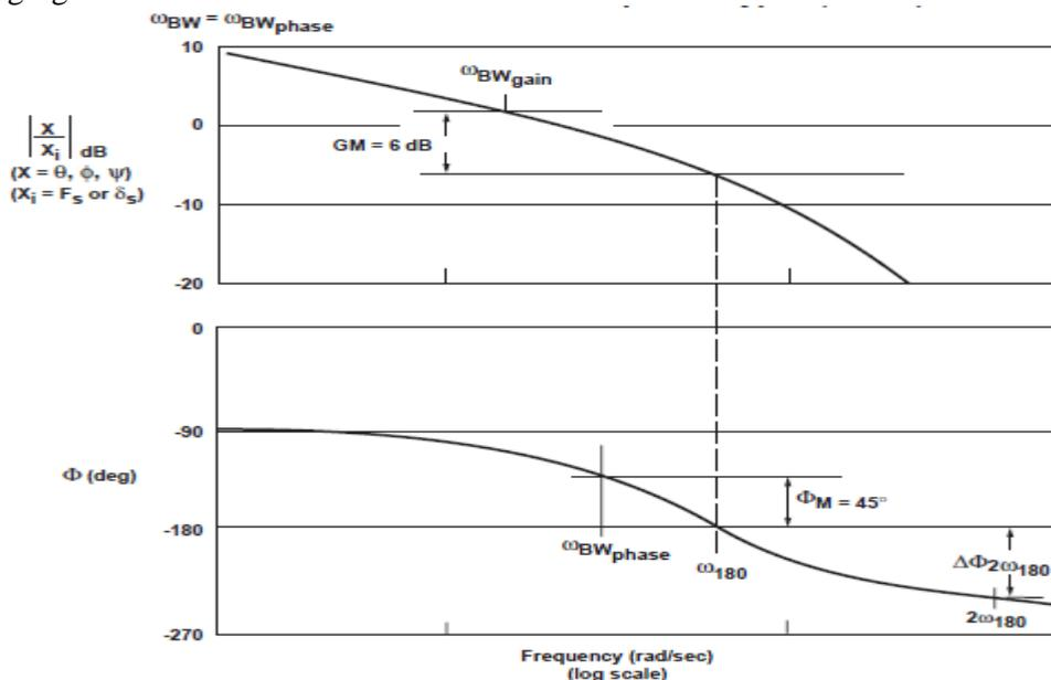
Figure 1. Definitions of bandwidth and phase delay
